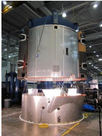
Dragon Trunk – Falcon 9 Second Stage Separation Qualification Test
