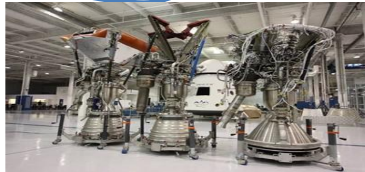
Merlin 1A (Falcon 1), Merlin 1C (Falcon 1 & 9) and Merlin 1C Vacuum (Falcon 9)
