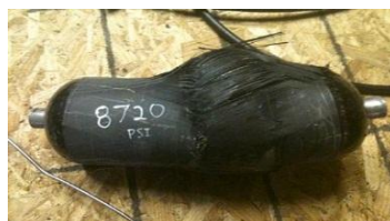
Development Test – Composite Overwrap Pressure Vessel Ultimate
