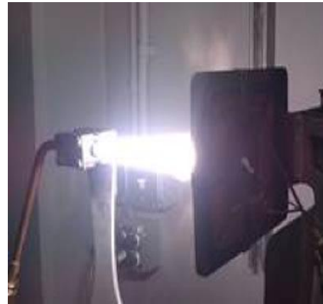
Merlin Nozzle Carbon Coating Development Test
