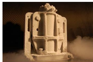
Thermal qualification of F9 separation system
